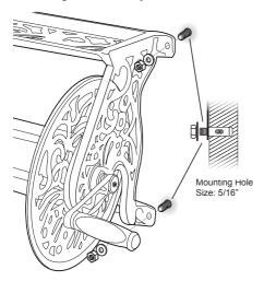
TIP: Remember to use the correct size and quantity of hardware to properly support the total weight of the unit. A standard 100' length of garden hose weighs approximately 15 lbs. Filled with water, the additional weight can exceed 20 lbs. The mounting hardware must be able to support the combined weight of the unit, garden hose, plus water.
